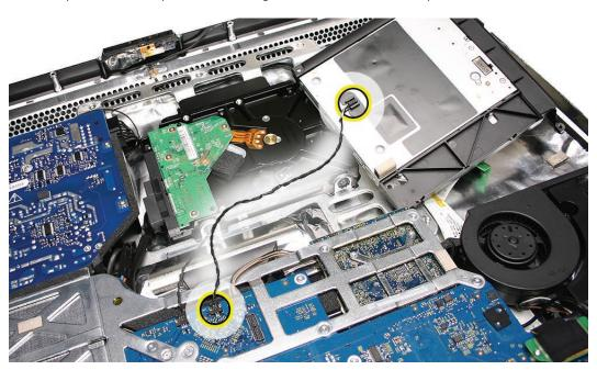
5. If you are replacing the optical drive, transfer the flex cable to the replacement drive. The replacement drive includes the plastic mounting brackets, sensor cable clip, slot-load bezel, and EMI gaskets.
